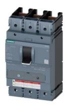
CIRCUIT BREAKER 3VA5 UL Frame 400 BREAKING CAPACITY CLASS M 35kA @ 480 V 3POLE, LINE PROTECTION TM230, FTAM, In=225A OVERLOAD PROTECTION IR=225A FIXED SHORT CIRCUIT PROTECTION Ii=5...10 x In W/O CONNECTION
