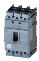
circuit breaker 3VA5 UL frame 125 breaking capacity class S 25kA @ 480 V 3-pole, line protection TM210, FTFM, In=90A overload protection Ir=90A fixed short-circuit protection li=10 x In cable connection on both sides
