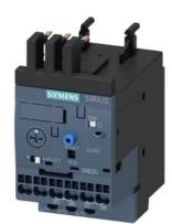
Overload relay 4...16 A Electronic For motor protection Size S00, Class 20E Contactor mounting Main circuit: Spring-type terminal Auxiliary circuit: Spring-type terminal Manual-Automatic-Reset
