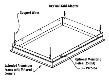
Installing a DGA in a drywall ceiling will provide a frame (grid) onto which you can lay-in any NEMA Type "G" troffer. This allows easier access to the plenum than when using flange trims with swing gate hangers.
