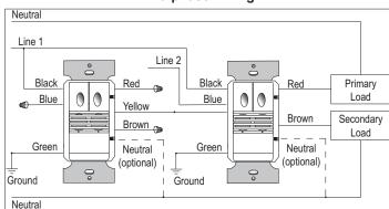
NOTE: Button 1 on any sensor controls load #1, and button 2 on any sensor controls load #2.
