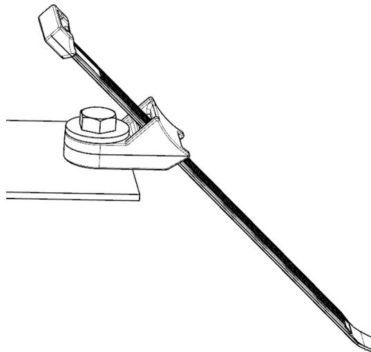
1.4 Loop the cable tie body around hoses, cables, wires, etc. and then thread the cable tie body through the head of the cable tie.
