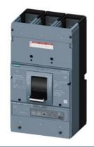
circuit breaker 3VA6 UL frame 1600 breaking capacity class C 100kA @ 480 V 3-pole, line protection ETU320, LI, In=1600A overload protection Ir=600A - 1600A short circuit protection Ii=1,5-7,5 x In w/o connection
