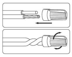
Use only on Copper to Copper (Cu/Cu) wire combinations. For use in dry locations only. Temperature rating: 105°C (221°F) maximum. 600 volts maximum building wire; 1000 volts signs or lighting fixtures.
