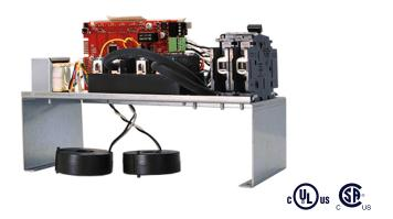
DCC-9-PCB is the electronic infrastructure that fits inside the DCC-9-BOX and allows the connection of an EV charger to the main feeder of a panel without affecting the load calculation.
