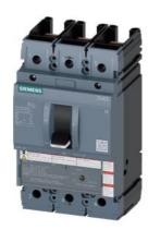
circuit breaker 3VA5 UL frame 250 breaking capacity class H 65kA @ 480 V 3-pole, line protection TM210, FTFM, In=60A overload protection Ir=60A fixed short circuit protection Ii=10 x In w/o connection
