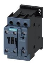
power contactor, AC-3e/AC-3, 38 A, 18.5 kW / 400 V, 3-pole, 110 V AC, 50 Hz / 120 V, 60 Hz, auxiliary contacts: 1 NO + 1 NC, screw terminal, size: S0
