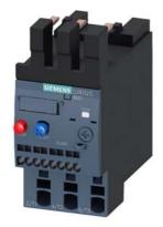
Overload relay 3.5...5.0 A Thermal For motor protection Size S0, Class 10 Contactor mounting Main circuit: Spring-type terminal Auxiliary circuit: spring-type terminal Manual-Automatic-Reset
