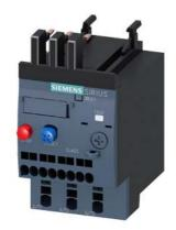
Overload relay 5.5...8.0 A Thermal For motor protection Size S00, Class 10 Contactor mounting Main circuit: Spring-type terminal Auxiliary circuit: spring-type terminal Manual-Automatic-Reset
