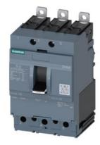
circuit breaker 3VA4 UL frame 125 breaking capacity class S 25kA @ 480 V 3-pole, line protection TM210, FTFM, In=40A overload protection Ir=40A fixed short-circuit protection Ii=10 x In clamp connection
