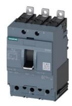
circuit breaker 3VA4 UL frame 125 breaking capacity class H 65kA @ 480 V 3-pole, line protection TM210, FTFM, In=80A overload protection Ir=80A fixed short-circuit protection Ii=10 x In clamp connection
