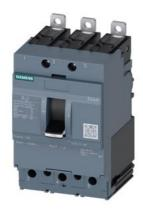
circuit breaker 3VA4 UL frame 125 breaking capacity class S 25kA @ 480 V 3-pole, line protection TM210, FTFM, In=90A overload protection Ir=90A fixed short-circuit protection Ii=10 x In clamp connection
