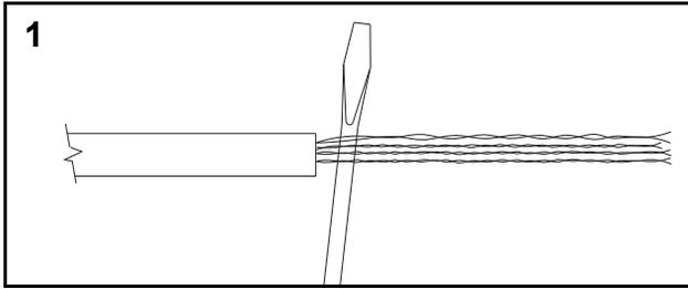
Remove 3" (76.2mm) of cable jacket and untwist pairs.
