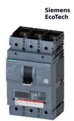
circuit breaker 3VA6 UL frame 400 breaking capacity class C 100kA @ 480 V 3pole, line protection ETU560, LSIG, In=400A overload protection Ir=160A ...400A short-circuit protection Isd=0.6..10x In, Ii=1.5..10x In N conductor protection opt. w. ext. CT; up to 160% ground-fault protection Ig=0.2... 1 x In, tg=0.05-0.8s nut keeper kit on both sides
