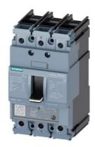
circuit breaker 3VA5 UL frame 125 breaking capacity class H 65kA @ 480 V 3-pole, line protection TM230, FTAM, In=100A overload protection Ir=100A fixed short-circuit protection Ii=5...10 x In cable connection on both sides
