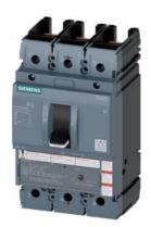
circuit breaker 3VA5 UL frame 250 breaking capacity class H 65kA @ 480 V 3-pole, line protection TM210, FTFM, In=15A overload protection Ir=15A fixed short circuit protection Ii=23,3 x In w/o connection
