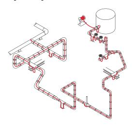
Starting from the end opposite the reel, tape the heating cable on the pipe at every foot, as shown in the figure above. If aluminum tape is used, apply it over the entire length of the heating cable after the cable has been secured with glass tape. Work back to the reel. Leave extra heating cable at the power connection, at all sides of splices and tees and at the end seal to allow for future servicing.
