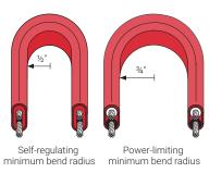
When positioning the heating cable on the pipe, do not bend tighter than  $\frac{1}{2}$ " for self-regulating cables and  $\frac{3}{4}$ " for power-limiting cables.
