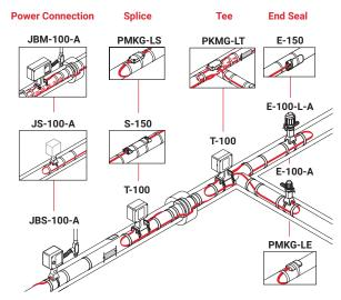
PMKG-LE, PMKG-LT, PMKG-LS are only approved for use with BTV and QTVR heating cables.
