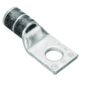
Copper HYLUGTM , Single Hole w/ Inspection Window,300, 1/2" Stud,17 index,White, Short Barrel,Electro- Tin Plated.
