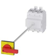
SENTRON, Switch disconnector 3LD, emergency switching-off switch, 3- pole, Iu=250 A, operating power / at AC-23 A 400 V: 132 kW, floor mounting with door coupling, knob-operated mechanism, red/yellow, 4-hole mounting of the handle
