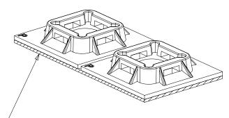
ADHESIVE BACKING: RUBBER BASED ADHESIVE PRESSURE SENSITIVE FOAM TAPE 0.04 [1.0] THICK WITH A PROTECTIVE LINER. MOUNT IS DESIGNED TO SUPPORT 0.50 lbs (227g) MAX. WEIGHT ON A CLEAN DRY SMOOTH SURFACE.
