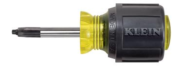
The Klein Tools Stubby #1 Square-Recess Tip Screwdriver has just a 1-1/2-Inch round-shank and works on most combination head receptacle and switch screws. Double wings inside handle provide solid, twist-resistant blade anchor. Cushion-Grip™ handles allow for greater torque and comfort.
