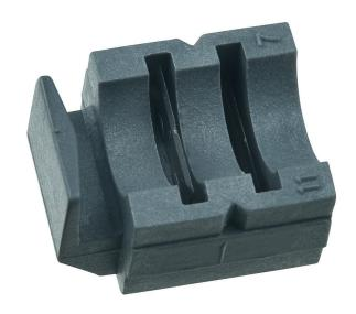
Strips Coaxial Cable, 2-level coaxial preparation of 5/16-Inch x 1/4-Inch. Pre-set cutting blades for precise and accurate stripping. Durable high-carbon steel cutting blades are ground and honed for long life. Patented V notch eliminates scoring of the center conductor. Designed for use with the following:
