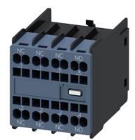
auxiliary switch, on the front, 1 NO + 3 NC, .1/.2, .1/.2, .1/.2, .3/.4, current path: 1 NC, 1 NC, 1 NC, 1 NO, spring-loaded terminal, for contactors 3RT2 and contactor relays 3RH2
