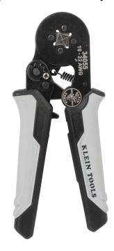
The full-cycle ratcheting ferrule crimper crimps 10-22 AWG ferrule terminals. This tool features four crimping dies that surround terminals 360 degrees for a high quality square shaped crimp. The unique design provides a low effort to crimp while maintaining a high terminal pull-off force. Built in ratchet ensures full-cycle crimping for a complete uniform crimp every time. Dual layer molded grips provide high level of comfort during use.
