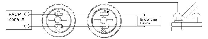
All wiring must be installed in compliance with the local Electrical Code using approved cable, AWG 18 minimum. Begin electrical connections by stripping approximately 1" (2.5 cm.) from the end of each wire. Insert the stripped end into the wire-retaining hole in the terminal bar, wrap clockwise around the terminal screw, and tighten. Circuit wiring must be broken at each terminal to ensure proper supervision.
