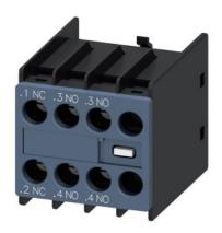
auxiliary switch, on the front, 2 NO + 1 NC, .1/.2, .3/.4, .3/.4, .-/-, current path: 1 NC, 1 NO, 1 NO, --, screw terminal, for contactors 3RT2 and contactor relays 3RH2
