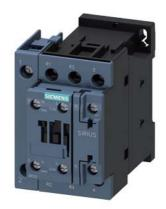
power contactor, AC-3, 25 A, 11 kW / 400 V, 4-pole, 110 V AC, 50 Hz / 120 V, 60 Hz, main contacts: 2 NO + 2 NC, auxiliary contacts: 1 NO + 1 NC, screw terminal, size:  $\pm$  S0
