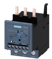
Overload relay 12.5...50 A Electronic For motor protection Size S2, Class 10E Contactor mounting Main circuit: Screw Auxiliary circuit: Screw Manual-Automatic-Reset
