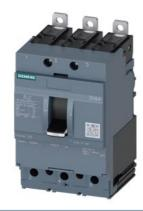
circuit breaker 3VA4 UL Frame 125 breaking capacity class H 65 kA @ 480 V 3-pole, line protection TM210, FTFM, In=100 A overload protection Ir=100 A permanently set short-circuit protection Ii=10 x In terminal connection
