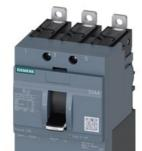
circuit breaker 3VA4 UL Frame 125 breaking capacity class S 25 kA @ 480 V 3-pole, line protection TM210, FTFM, In=50 A overload protection Ir=50 A permanently set short-circuit protection Ii=10 x In terminal connection
