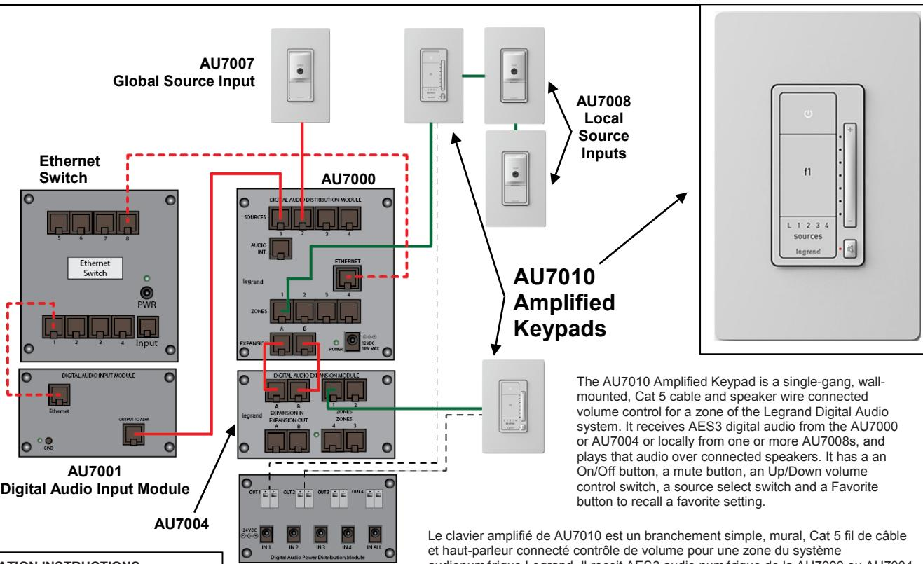
The AU7010 Amplified Keypad is a single-gang, wall-mounted, Cat 5 cable and speaker wire connected volume control for a zone of the Legrand Digital Audio system. It receives AES3 digital audio from the AU7000 or AU7004 or locally from one or more AU7008s, and plays that audio over connected speakers. It has an On/Off button, a mute button, an Up/Down volume control switch, a source select switch and a Favorite button to recall a favorite setting.
