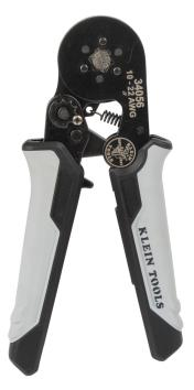
The full-cycle ratcheting ferrule crimper crimps 10-22 AWG ferrule terminals. This tool features six crimping dies that surround terminals 360 degrees for a high quality hex shaped crimp. The unique design provides a low effort to crimp while maintaining a high terminal pull-off force. Built in ratchet ensures full-cycle crimping for a complete uniform crimp every time. Dual layer molded grips provide high level of comfort during use.
