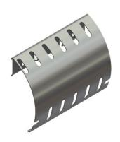
The Standard Dropout (SDO) offers stronger cable support and creates a seamless transition for your cables over the side of your wire mesh tray without any cutting. This allows you to safely transition your cables as they exit the tray over the siderail while maintaining all the strength and support of your wire mesh.
