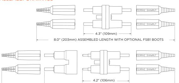
5.6" (142mm) ASSEMBLED LENGTH 8.6" (218mm) ASSEMBLED LENGTH
