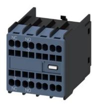
auxiliary switch, on the front, 1 NO + 1 NC, .1/.2, .3/.4, --/--, current path: 1 NC, 1 NO, --, --, spring-loaded terminal, for contactors 3RT2 and contactor relays 3RH2
