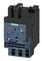
Overload relay 0.32...1.25 A Electronic For motor protection Size S0, Class 20 Contactor mounting Main circuit: Spring-type terminal Auxiliary circuit: Spring-type terminal Manual-Automatic-Reset
