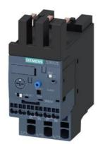
Overload relay 0.32...1.25 A Electronic For motor protection Size S0, Class 10E Contactor mounting Main circuit: Spring-type terminal Auxiliary circuit: Spring-type terminal Manual-Automatic-Reset
