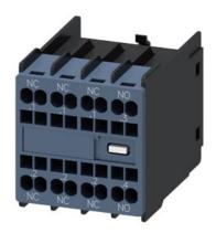
auxiliary switch, on the front, 1 NO + 3 NC, .1/.2, .1/.2, .1/.2, .3/.4, current path: 1 NC, 1 NC, 1 NO, spring-loaded terminal, for contactors 3RT2 and contactor relays 3RH2
