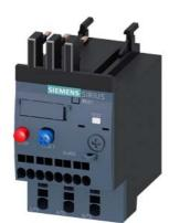
Overload relay 5.5...8.0 A Thermal For motor protection Size S00, Class 10 Contactor mounting Main circuit: Spring-type terminal Auxiliary circuit: spring-type terminal Manual-Automatic-Reset
