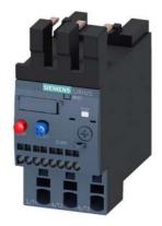
Overload relay 23...28 A Thermal For motor protection Size S0, Class 10 Contactor mounting Main circuit: Spring-type terminal Auxiliary circuit: spring-type terminal Manual-Automatic-Reset
