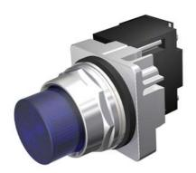
30mm Command/52, Chrome Finish Heavy Duty, Watertight/Oiltight Complete Metal Unit Illuminated Indicator Light Transformer type, 120V AC LED Lamp, BA9s Plastic Lens, Blue UL Listed, CSA Certified NEMA 1,3,3R,4,4X,12,13 & Automotive Standards
