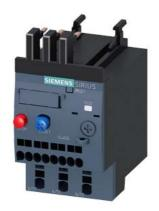
Overload relay 11...16 A Thermal For motor protection Size S00, Class 10 Contactor mounting Main circuit: Spring-type terminal Auxiliary circuit: spring-type terminal Manual-Automatic-Reset
