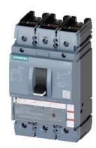
circuit breaker 3VA5 UL Frame 250 breaking capacity class M 35 kA @ 480 V 3-pole, line protection TM230, FTAM, In=200 A overload protection Ir=200 A permanently set short-circuit protection Ii=5...10 x In cable connection on two sides
