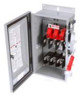
Siemens Low Voltage Circuit Protection Heavy Duty Safety Switch. 3-Pole 3-Fuse Fused in a type 12 industrial enclosure. Rated 600VAC (100A).
