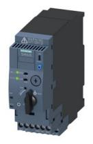
SIRIUS Compact load feeder DOL starter 690 V 24 V AC/DC 50...60 Hz 0.1...0.4 A IP20 Connection main circuit: plug-in, without terminals Connection auxiliary circuit: screw terminal
