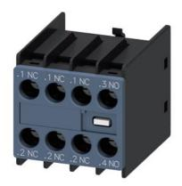
auxiliary switch, on the front, 1 NO + 3 NC, .1/.2, .1/.2, .3/.4, current path: 1 NC, 1 NC, 1 NC, 1 NO, screw terminal, for contactors 3RT2 and contactor relays 3RH2
